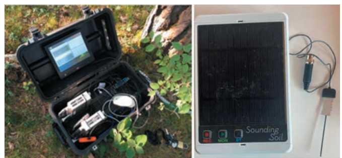
Figure 9 Sounding Soil bioacoustics equipment. To the left is the Sounding Soil in the field (Maeder et al., 2019), to the right is the main body and the probe sensors.
